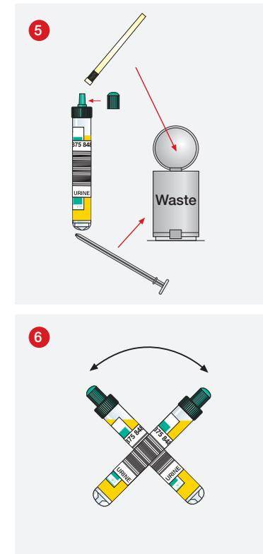
Remove the aspiration tip, **break off the piston rod and discard both.** Replace the stopper.
