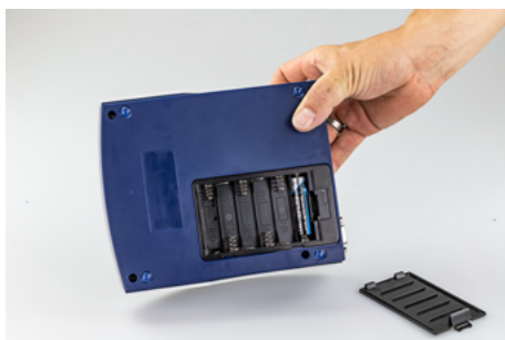
Pic 17: Battery compartment
